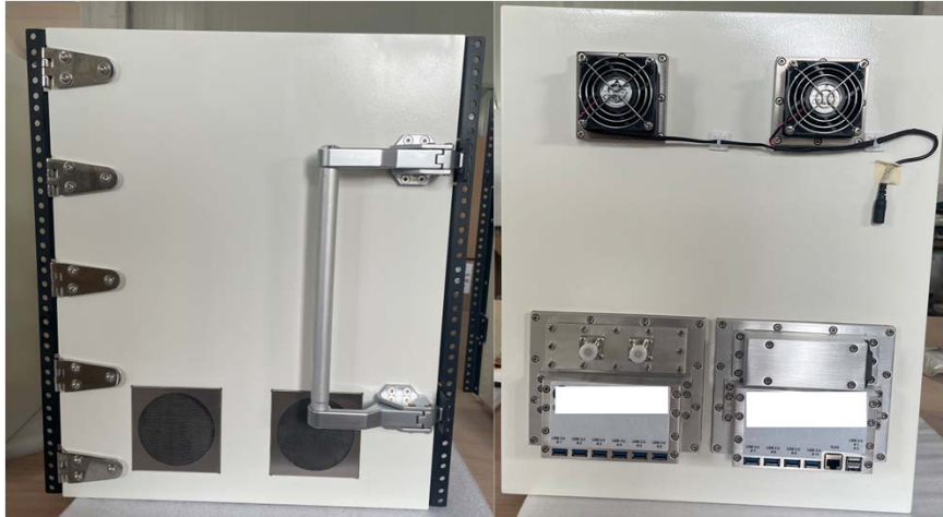
12U RF shielding cabinet for 19' Rack system
